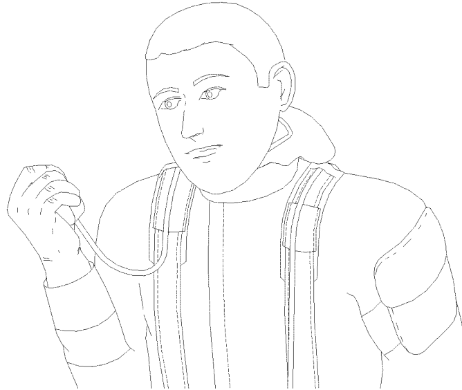
Figure 077-3-25. Checking Remote Pressure Indicator
