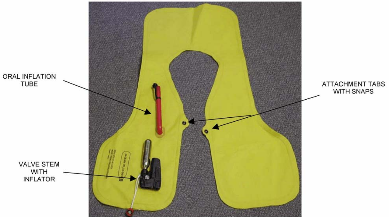
Figure 077-2-9. Inflatable Bladder for MK-1 Vest Type Life Preserver
