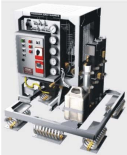
Figure 077-3-35. High Pressure Breathing Air Compressor
